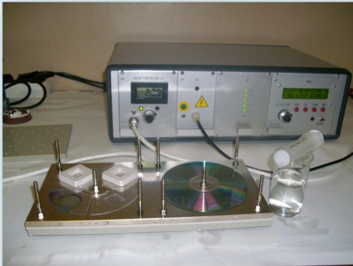
Specimens of CDs/DVDs loaded for chemical and electrochemical etching in the Laboratory of Dosimetry and Radiation Protection at the Faculty of Physics, Sofia University
