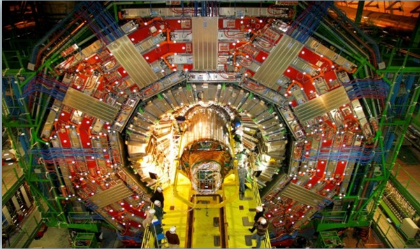
The CMS detector. Installation of the Central Tracker
